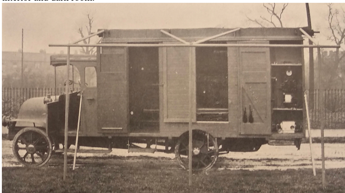
Figure 7 Austin mobile x-ray van c. 1917, showing tent framework and side access to interior and dark room.
