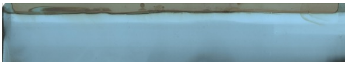
Figure 2: X-ray film showing undeveloped region at top due to incorrect chemical levels, and damage to emulsion layer on left side caused by a channel hanger.
